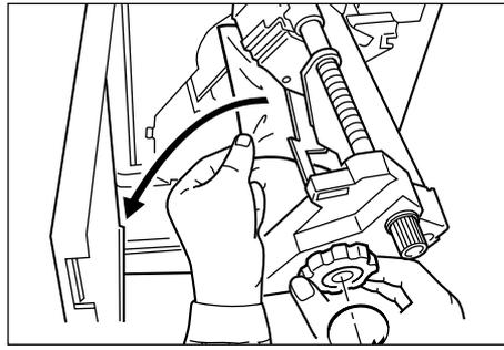
3. Turn the knob to release the stitcher and remove jam paper.
