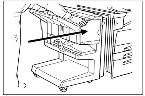
5. Reinstall the waste punch box by aligning its locking tab with the groove in the finisher.
