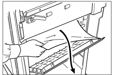
3. Turn the knob clockwise to feed the jam paper to the saddle stitcher tray section and remove the paper.
