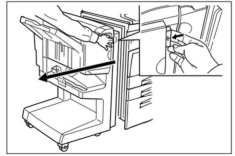
1. Push the lock release button and release the finisher from the machine body as shown.
