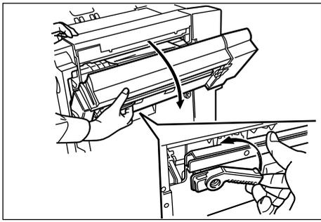
2. When the reverse unit is installed, raise the lever to open the reverse unit.
