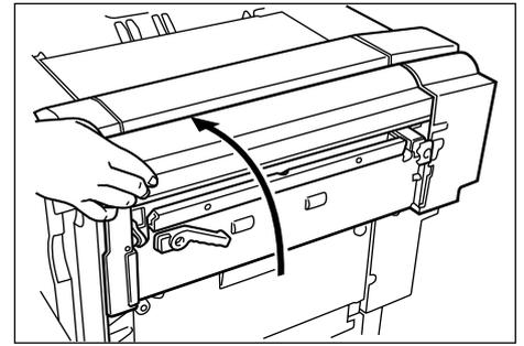
5. When the reverse unit is installed, close it.
