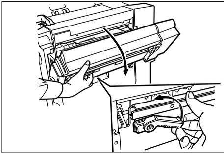
3. When the reverse unit is installed, raise the lever to open the reverse unit.
