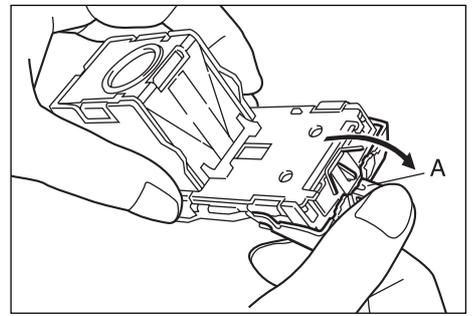
5. Open the plate on the holder by pushing the tab "A".
