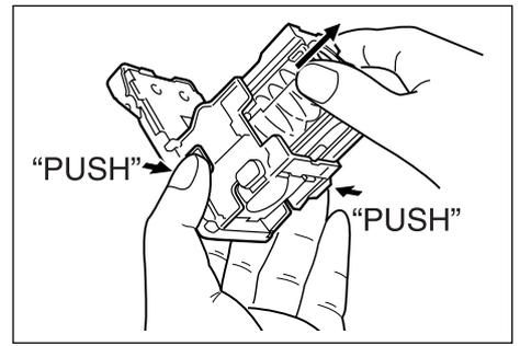
5. Depress the right and left "PUSH" marks to release the staple retainer.
