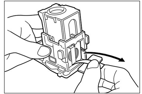
8. Peel the tape securing the staples to the staple case by pulling it.
