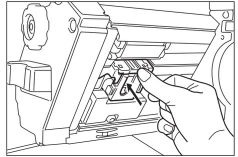
8. Reinstall the staple holder and press it until it is locked.
