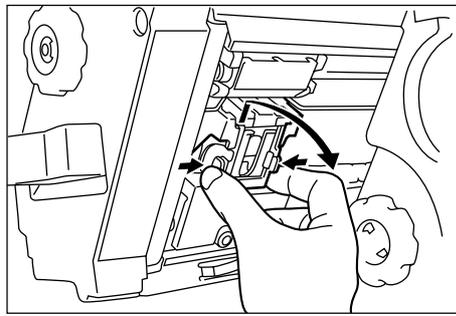
4. Remove the staple holder by lifting slightly and pulling it while pressing the right and left buttons on the staple holder.
