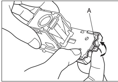
7. Close the protective faceplate by pushing the tab "A".
