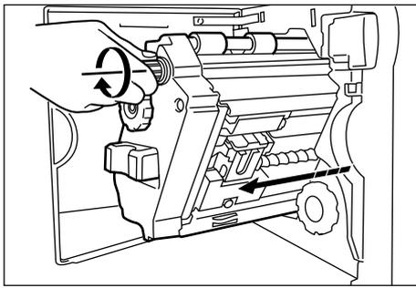
3. Turn the knob clockwise until the staple holder section reaches the front-most position.
