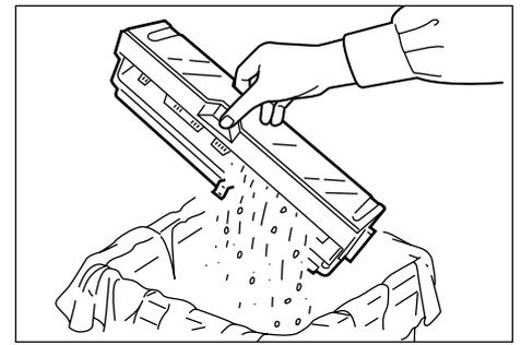
4. Dispose of the punch waste appropriately.
