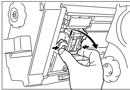
4. Remove the staple holder by lifting slightly and pull out the cartridge while pressing the right and left buttons on the staple holder.
